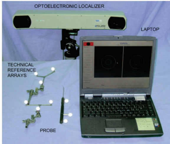
Fig. 1. Navigation system: optical localizer (Polaris, NDI, Canada) and laptop. Tracked markers and probe.
