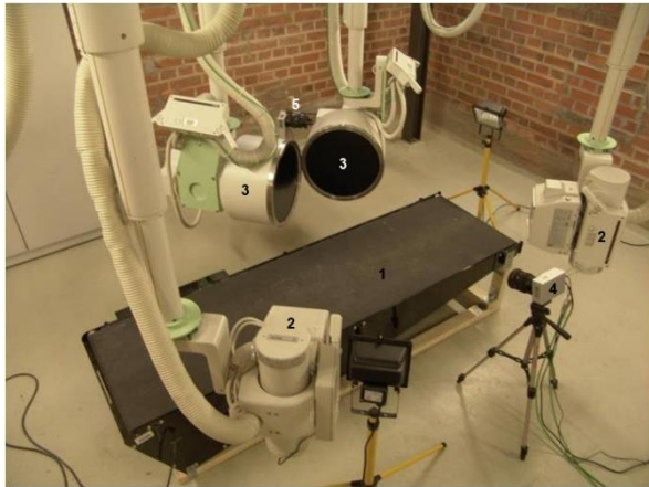
Fig. 2. Setup for high-speed bi-planar fluoroscopic kinematography. (1): treadmill; (2): x-ray tube assembly; (3): image intensifier; (4): digital high-speed video camera for live image capturing; (5): digital high-speed video cameras coupled to the image intensifier. The inter-beam angle is \sim 60^\circ and the x-ray source-to-image intensifier distance 1.4 m.
